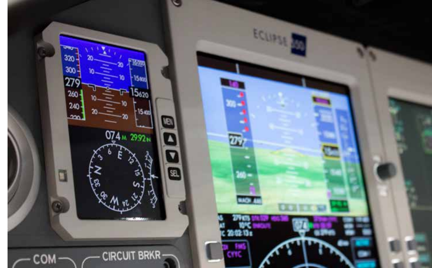
Above: The Standby Display Unit on the pilot side next to a PFD with optional synthetic vision.
